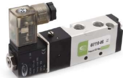
5 Way Pneumatic Solenoid Air Valve 2 Position PT1/8" Internally Piloted Acting Type - 4V110-06 DC24V
